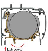
3. The cradle is lowered into place and secured along the span with jack screws.
