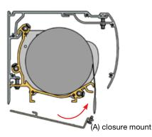
4. The closure mount (A) is hooked into the bottom of the cradle and then secured along the span with screws.
