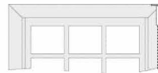
2. Measure ordered shade opening (Back-of-bracket to back-of-bracket)
